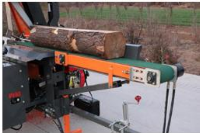
Automatic feeding conveyor system
