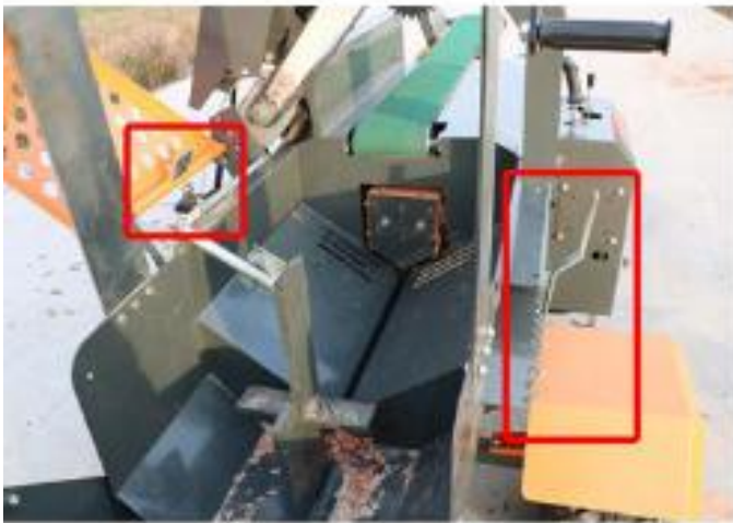
Automatic protection device
