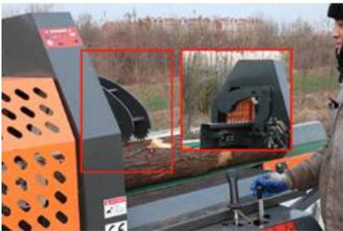
Hydraulic automatic log clamping
