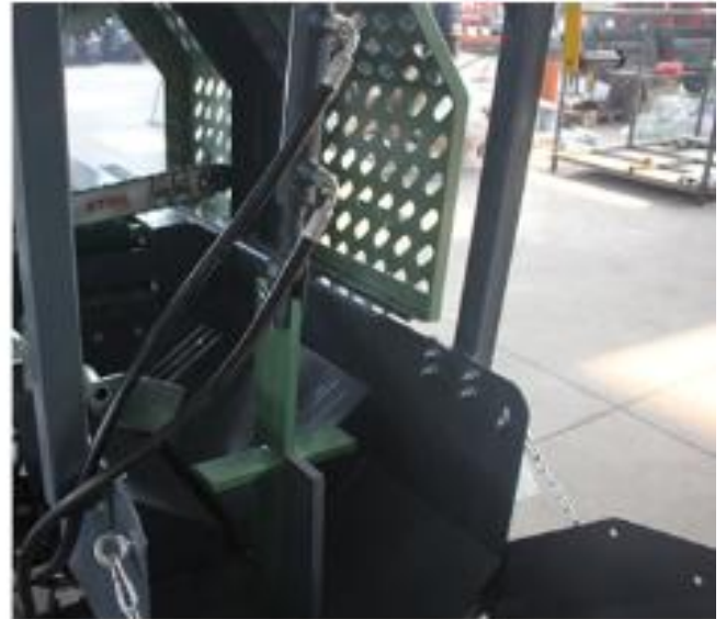
Splitting Blade is Adjustable
